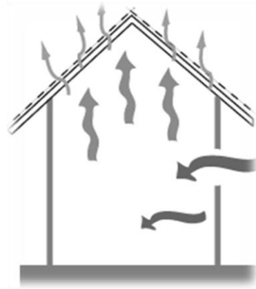
Figure 3: Good Ventilation System in the Traditional Maldivian House
