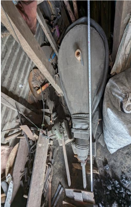
Fig. 3. Bellows made of rubber
