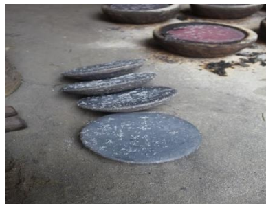
Fig. 32. Bun shape bronze metal ingot
